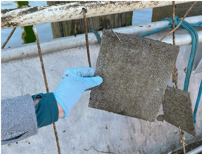
Figure 12. Close-up of passive sampler in mesh bag following retrieval
