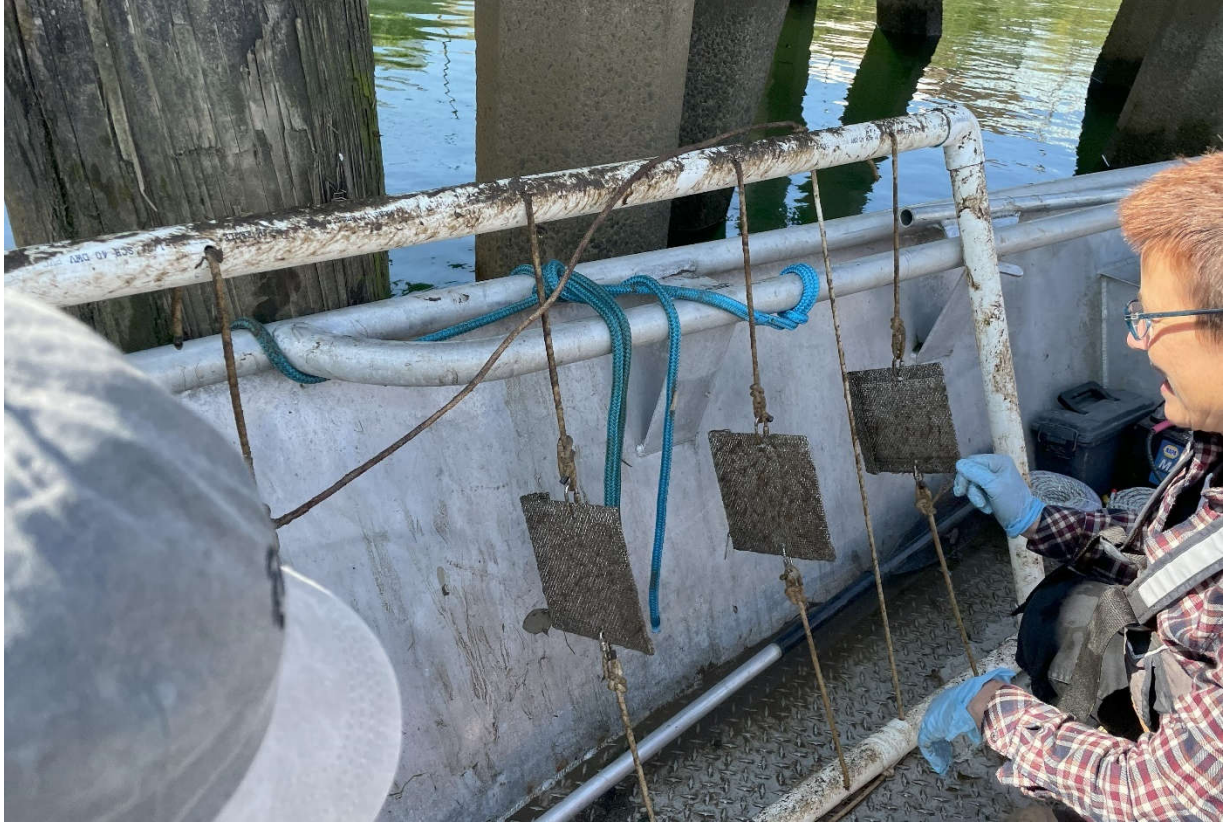
Figure 11. Retrieval of passive sampler frames
