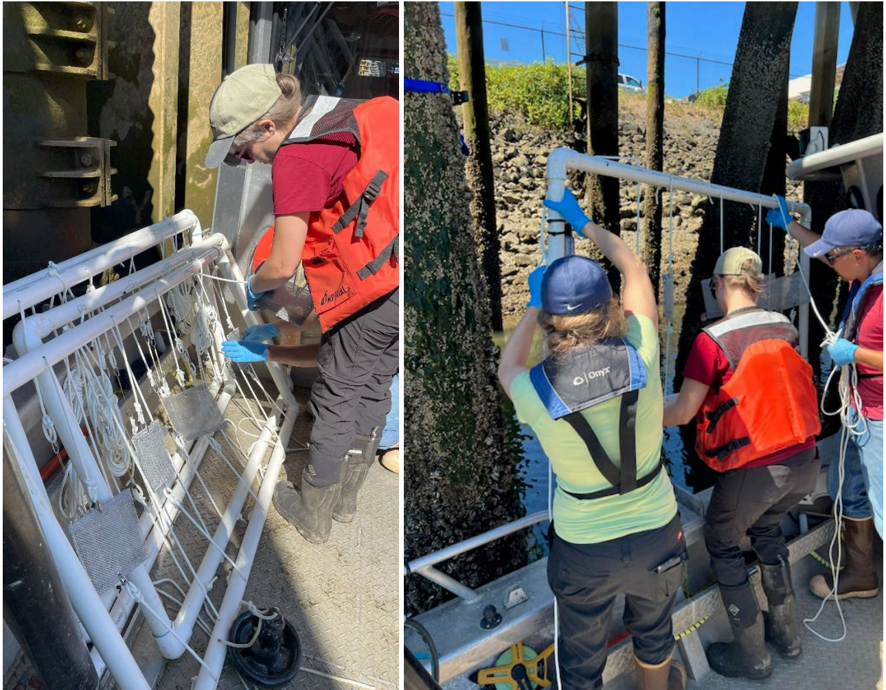
Figure 10. Preparation of passive sampler frames and deployment
