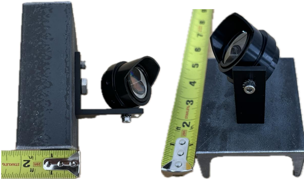
Figure 9: Trimble 25mm monitoring prisms on bracket.
