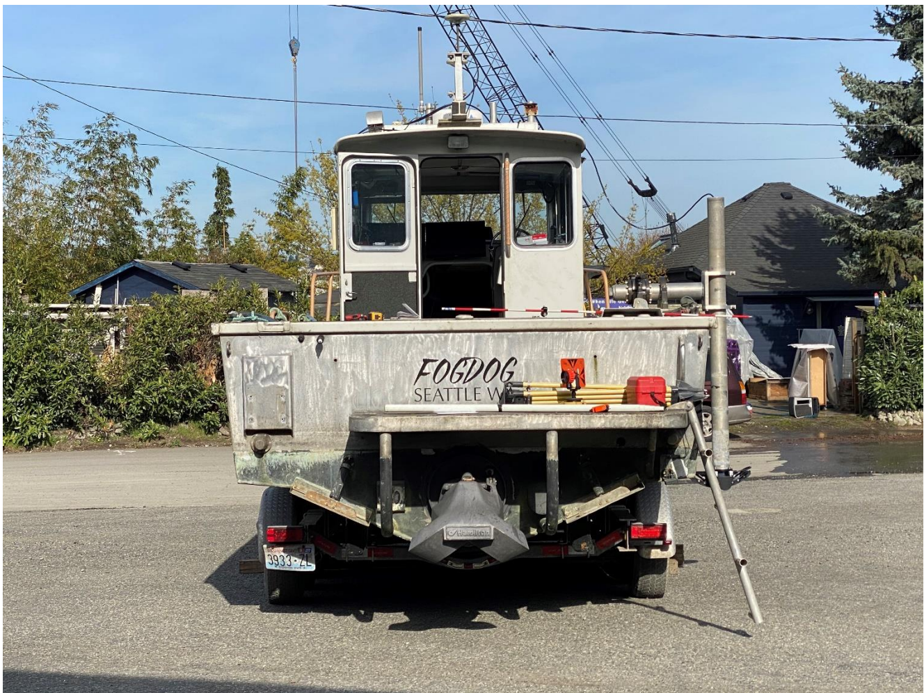
Figure 9. Man Overboard Recovery Zone at Starboard Swim Step
