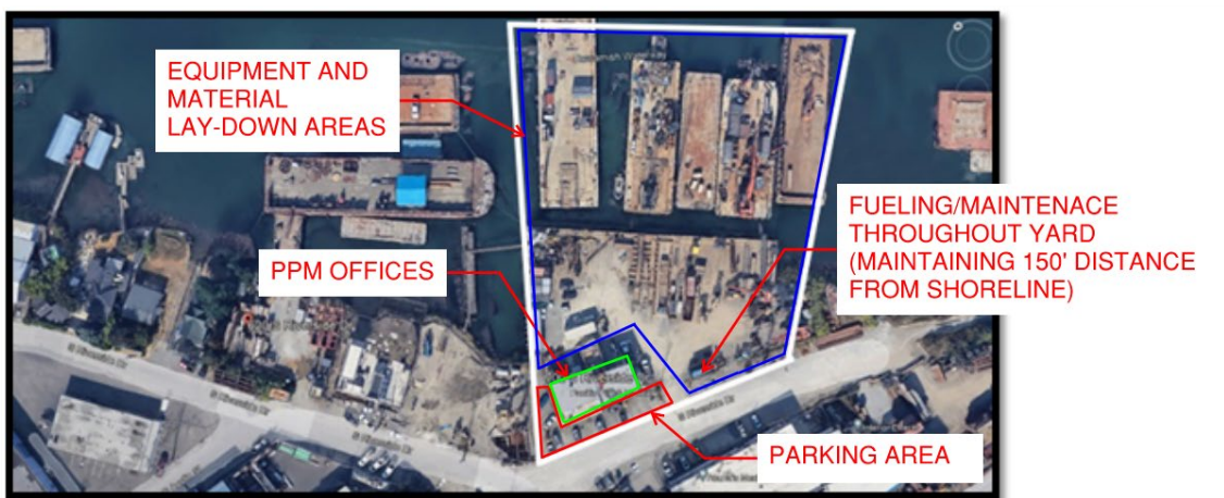
Figure 1- PPM permanent lay-down yard and offices.
