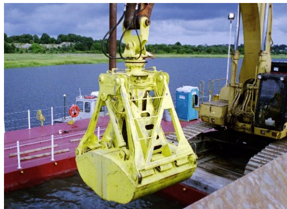
Articulated bucket (horizontal profile grab)
