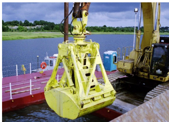
Articulated environmental bucket (horizontal profile grab)
