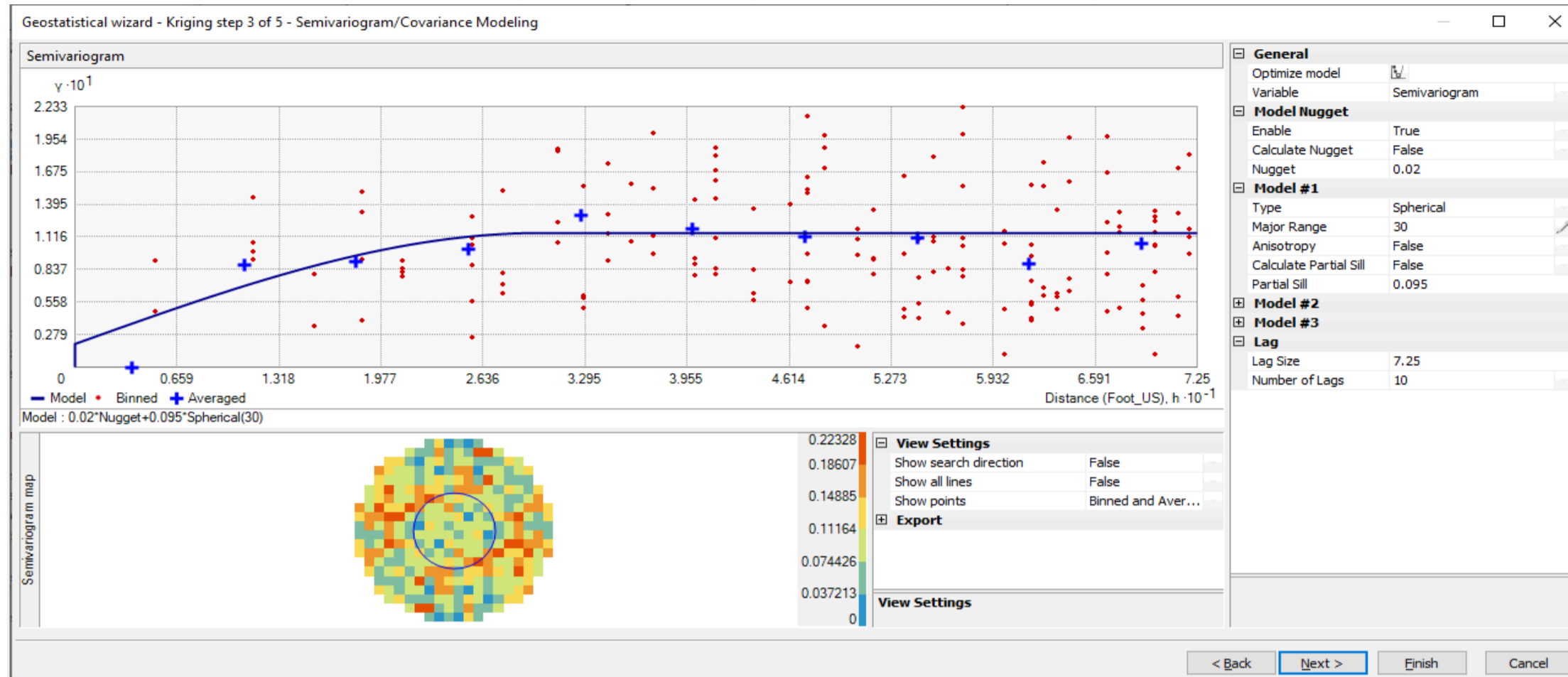
Figure A.4.2-1 Phase III surface sediment and subsurface sediment semivariogram plots and spatial correlation models
