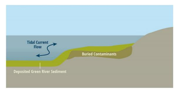
**Enhanced natural recovery**, which uses a thin layer of clean sand to speed up the natural recovery process.
