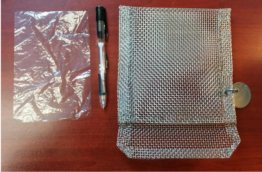
Figure 4-3 Polyethylene Sampler and Holder for Surface Water Deployment
