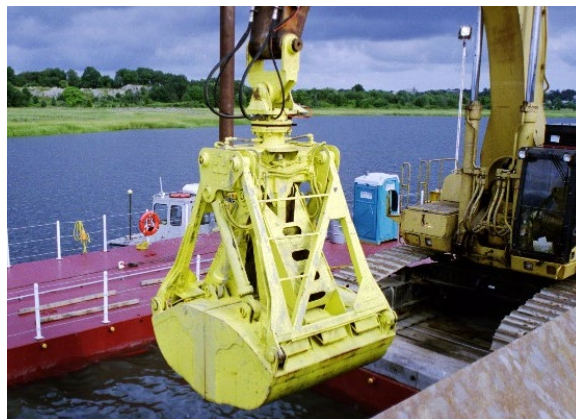
Articulated bucket (Horizontal Profile Grab)
