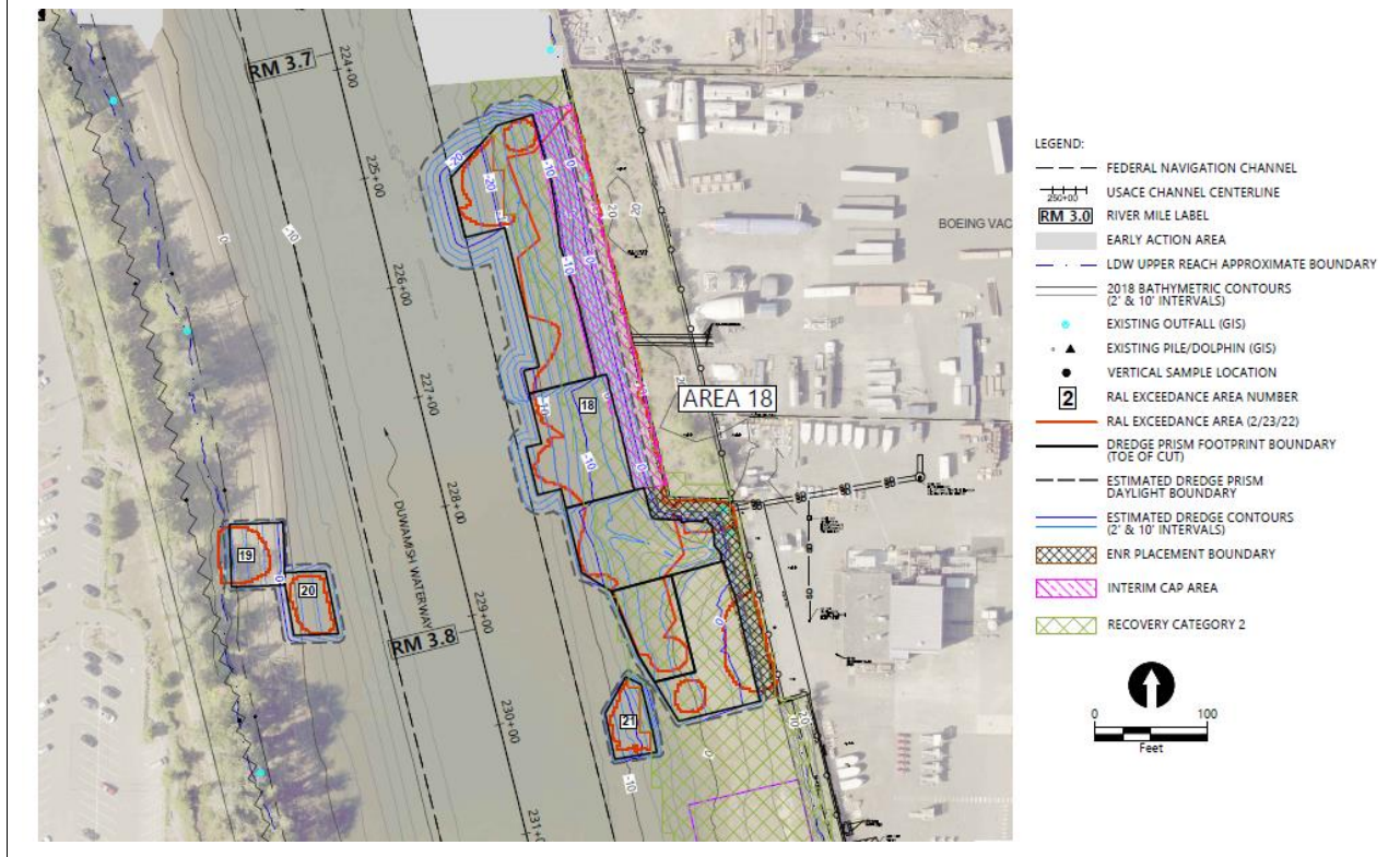
Figure G-1 Area 18—Partial Dredge and Cap Area
