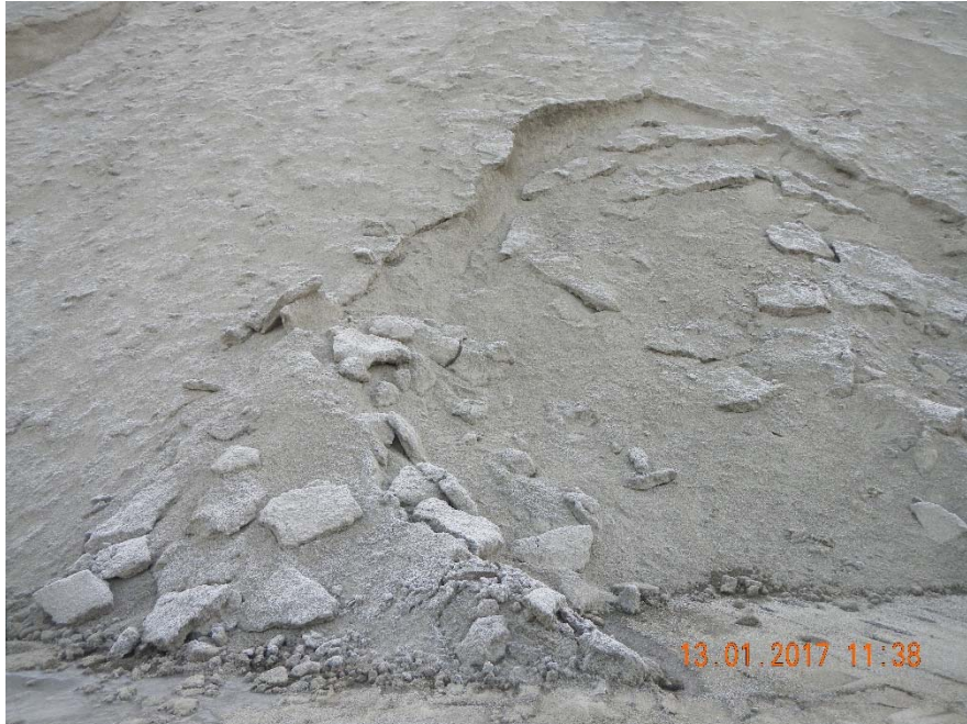
Photo 2-A: Sand ENR stockpile at the Cal-Portland's Dupont facility. Note the blocks of frozen sand. These blocks of frozen sand made loading difficult.
