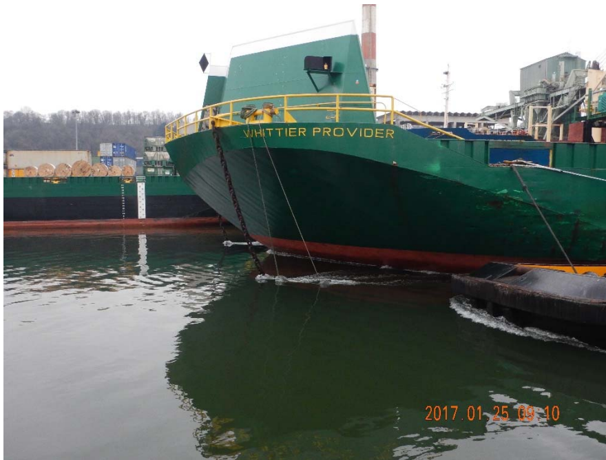
Photo 1-A: AML barge Whittier Provider being taken upstream with bridle chains hanging from bow.
