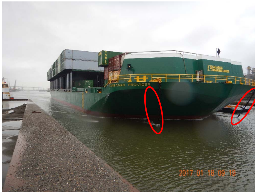
Photo 1-B: Barge traffic on the waterway passing on the east side of the material barge. Note the tow bridle hanging down into the water from the bow (circle in red).
