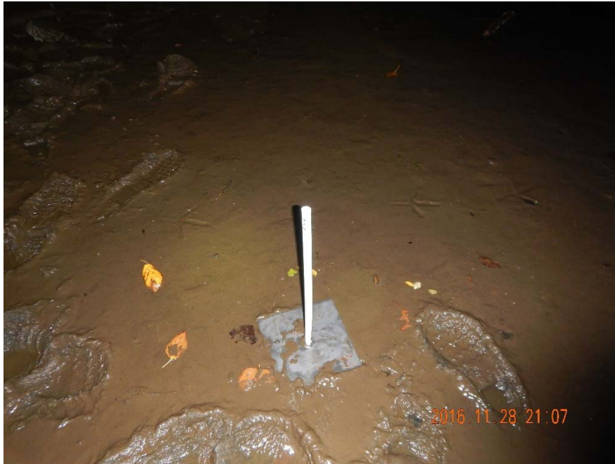
Photo 1-A: Example of a stake placed in the intertidal plot that will be used to measure the cap thickness. All stakes extended 18 inches above the mudline.
