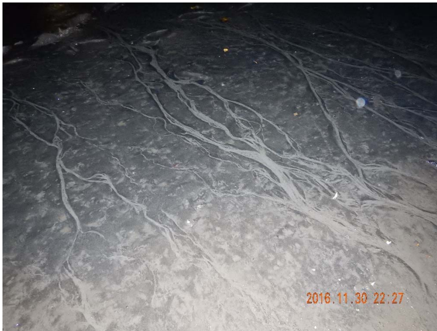
Photo 1-B: Activated carbon settled outside of the placement plot. This is approximately 15 feet outside of the placement area.
