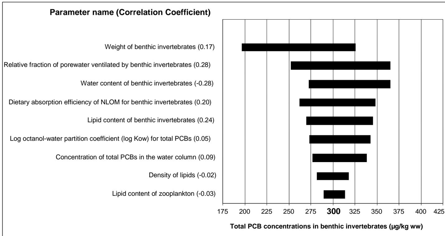
**Figure D.6-1. Results of the NRS analysis for benthic invertebrates**
