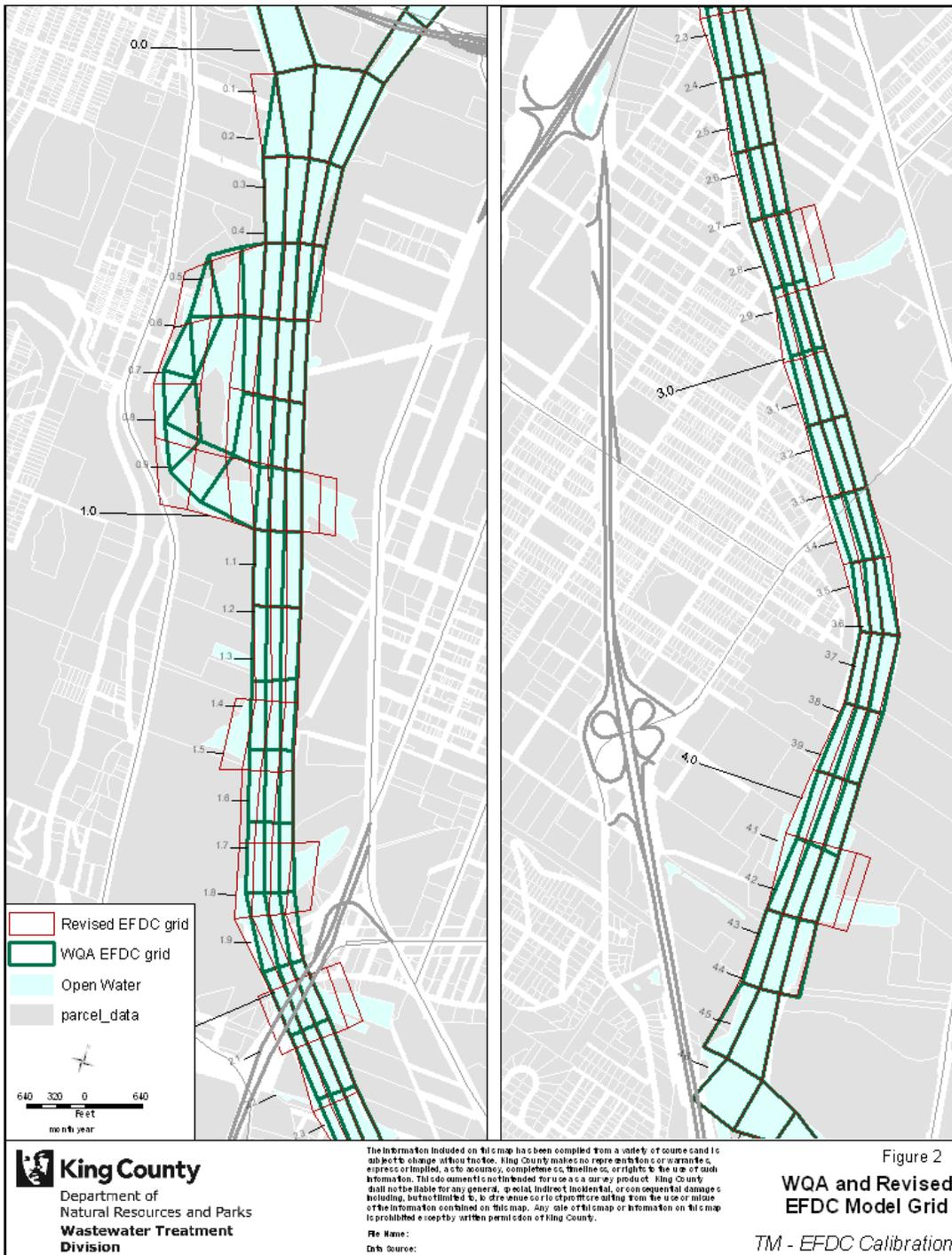
Figure 2. Comparison of original WQA model grid and revised model grid. Cells representing slips were sized to match surface area and depth of the slips.
