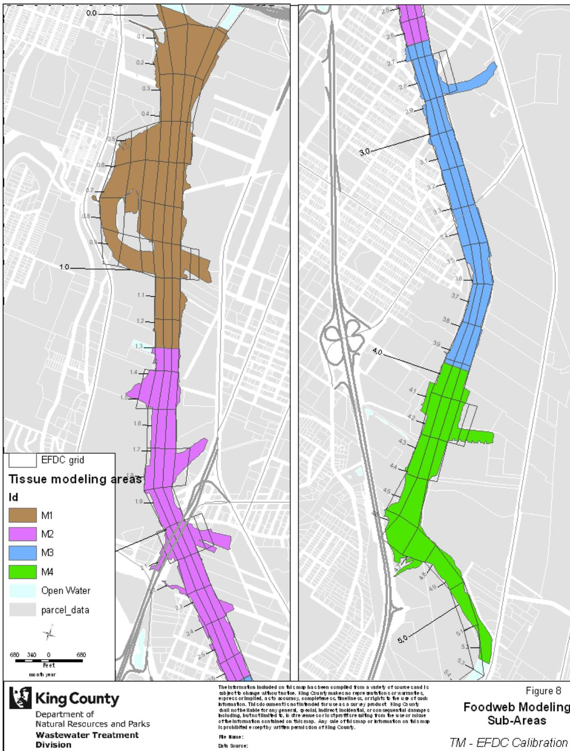
Figure 8. The EFDC grid and the four tissue modeling areas used in the LDW Food Web Model.
