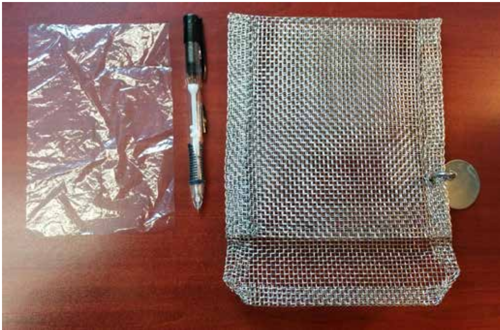
Figure 4-5. Polyethylene sampler and holder for surface water deployment
