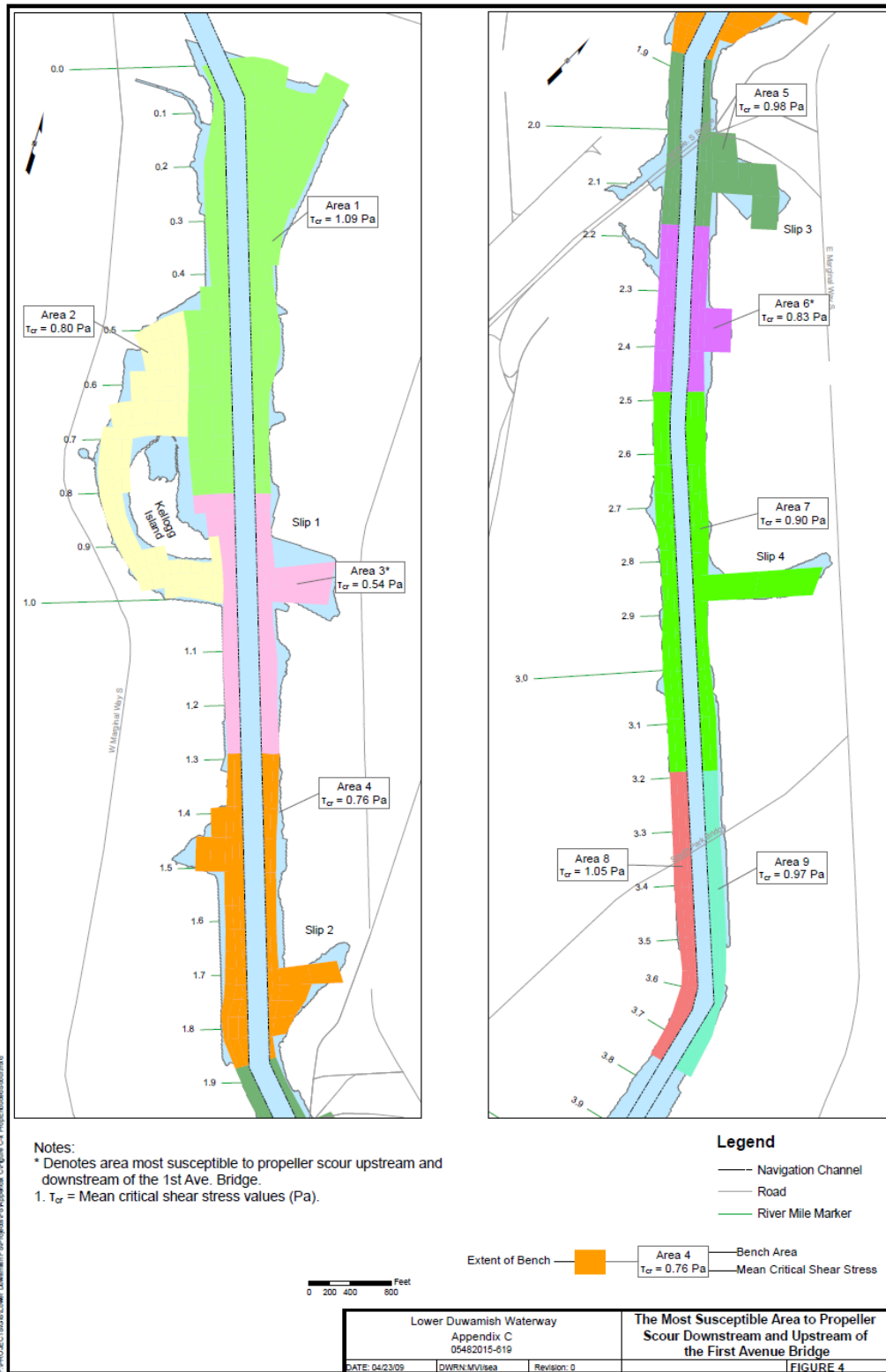
Figure 4 The Most Susceptible Area to Propeller Scour Downstream and Upstream of the First Avenue Bridge
