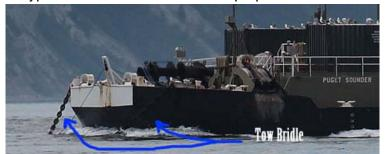
crew led to the hypothesis that when large, ocean going barges enter the Duwamish Waterway, they lower and drag their bow mounted tow bridles as they are pushed by tugs up the waterway.
