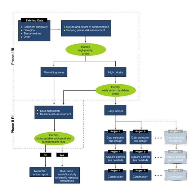
Figure 2. Flowchart of tasks for the Lower Duwamish Waterway RI/FS
