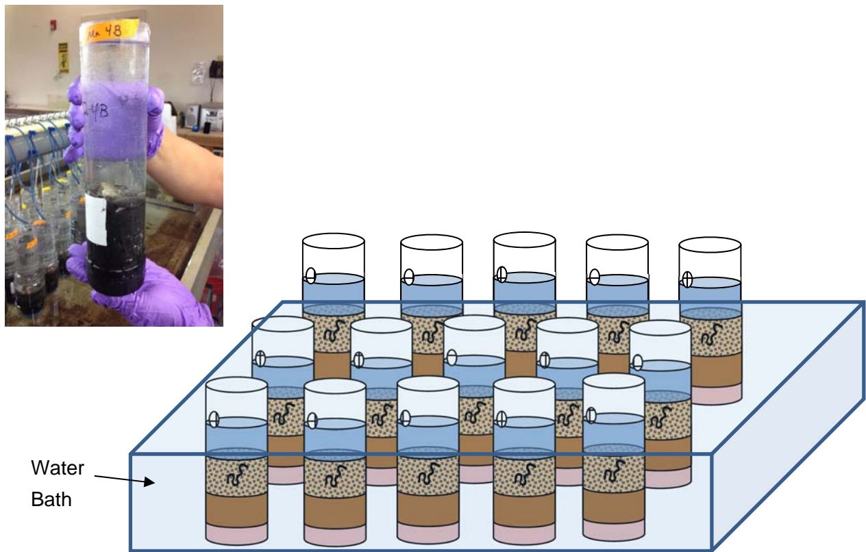
Figure 3.3. Schematic of an Array of Cores in the Water Bath and an Example of a Test Core (note: photo is for illustrative purposes only and is not to the size and scale proposed for this experiment).
