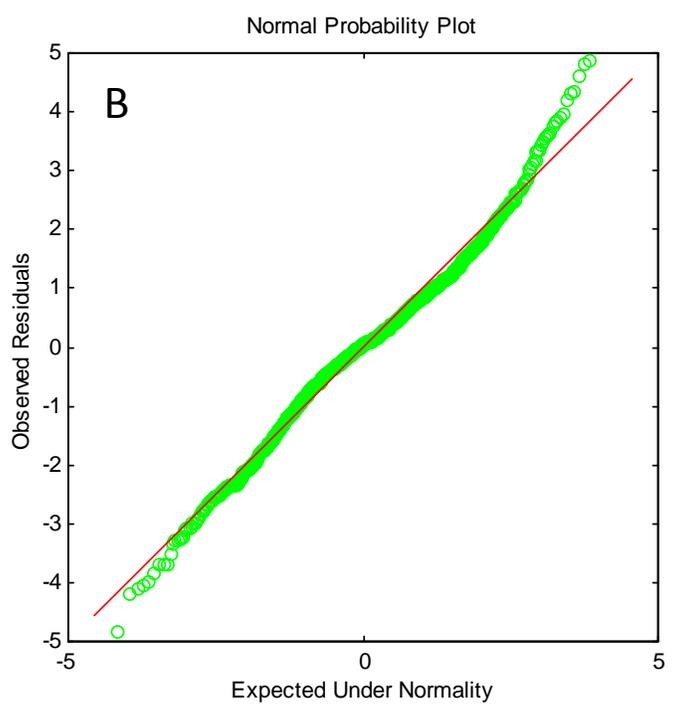
Figure 2. Histogram of residuals of log(PCB) with fitted normal distribution (panel A) and normal probability plot for residuals (panel B). Residuals are similar to a normal distribution ( $p > 0.10$ )
