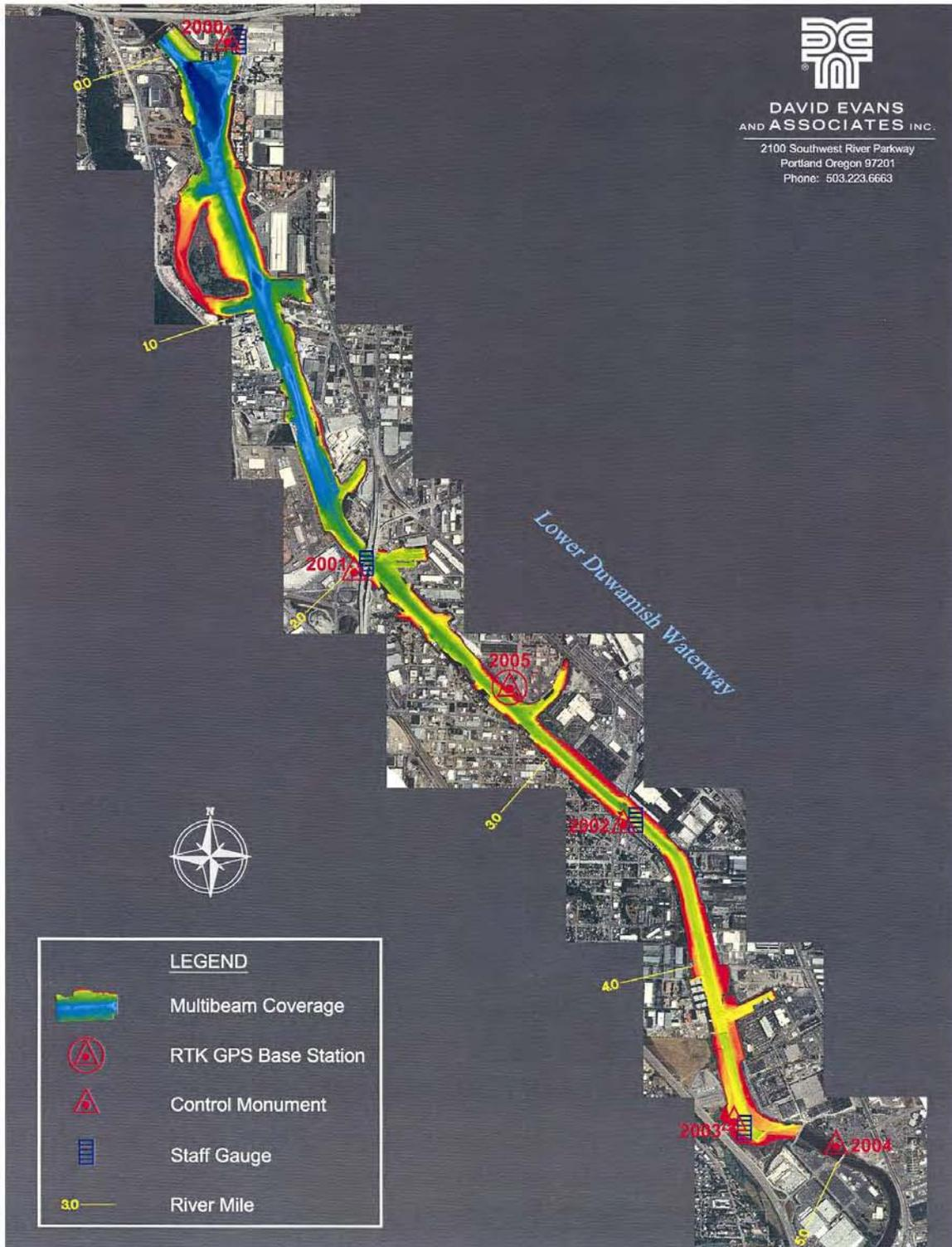
**Figure 1. Coverage of bathymetric survey of the Lower Duwamish Waterway**
