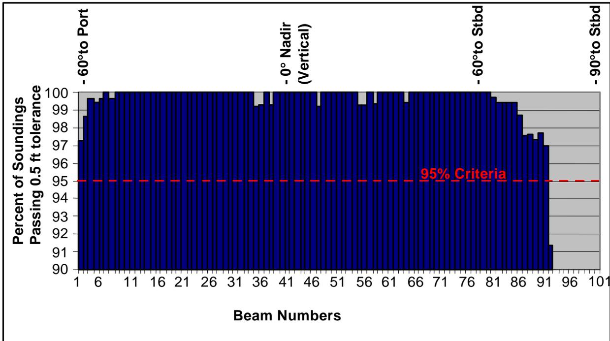
**Figure 6. Cross-line analysis using a 0.5 ft tolerance at a 95% confidence level**
