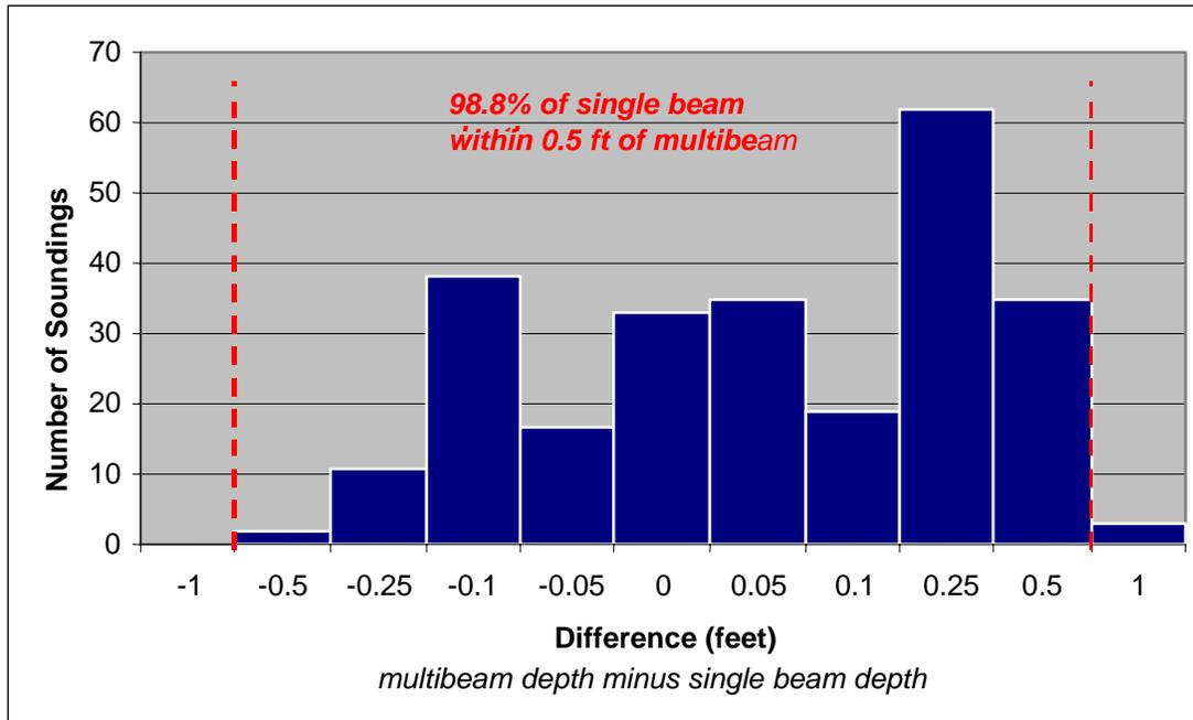
**Figure 7. Results of single beam comparison to outer multibeam data**
