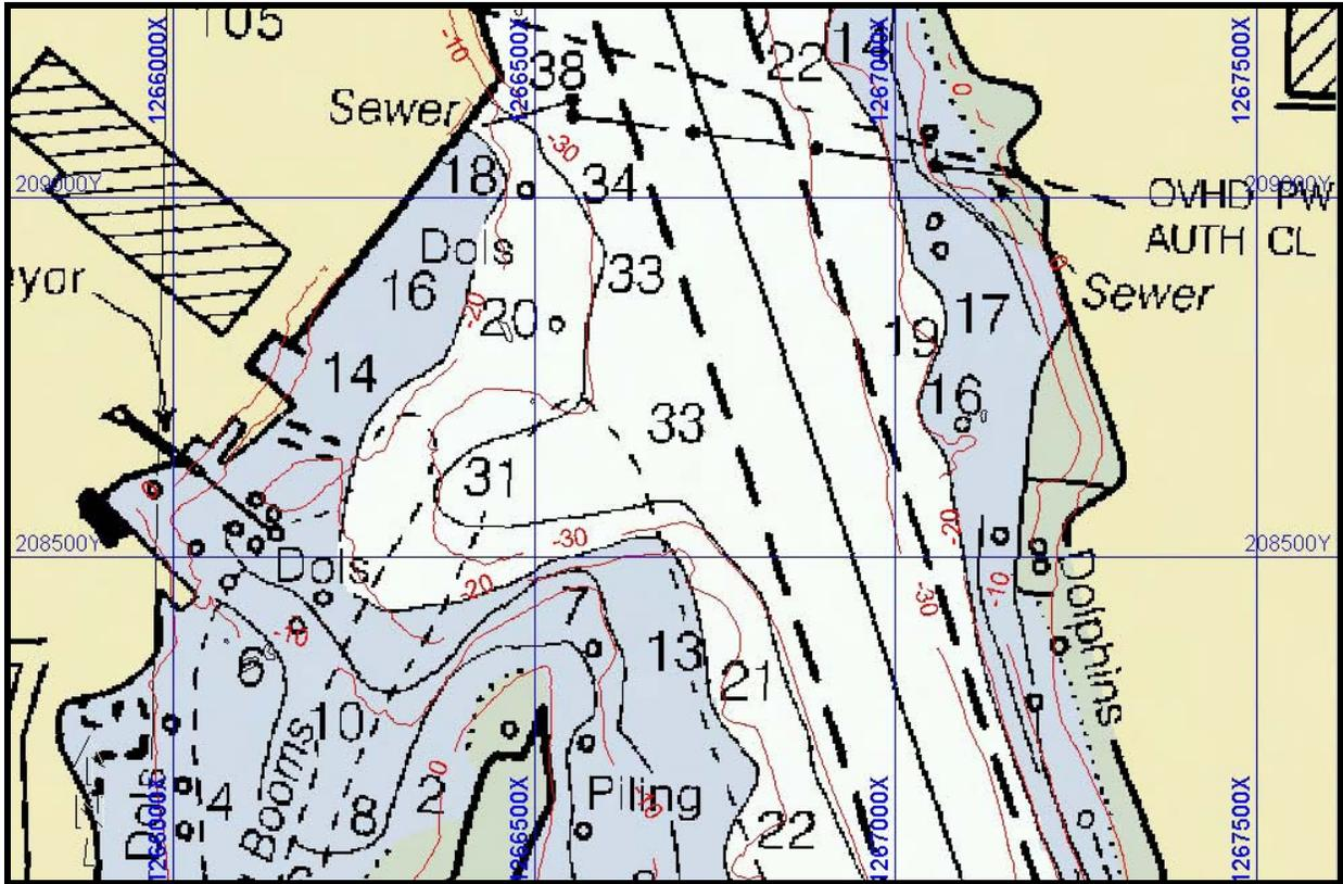
**Figure 5. Comparison of multibeam contours to NOAA chart**
