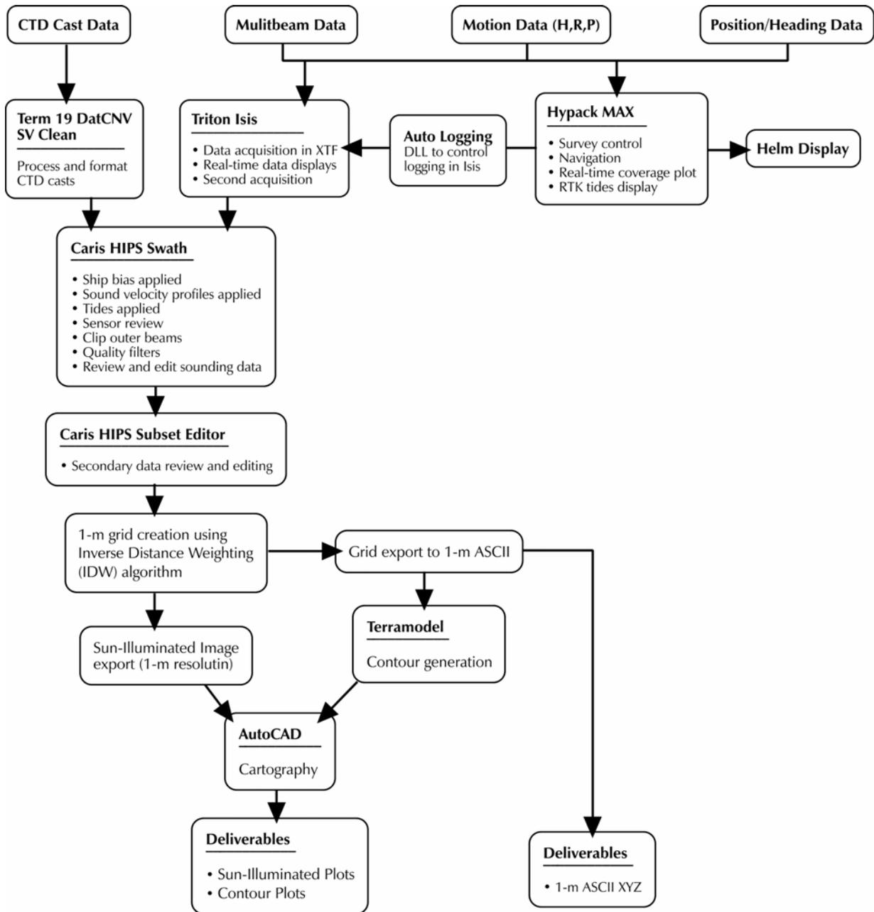
**Figure 2. Multibeam data acquisition and processing flowchart**
